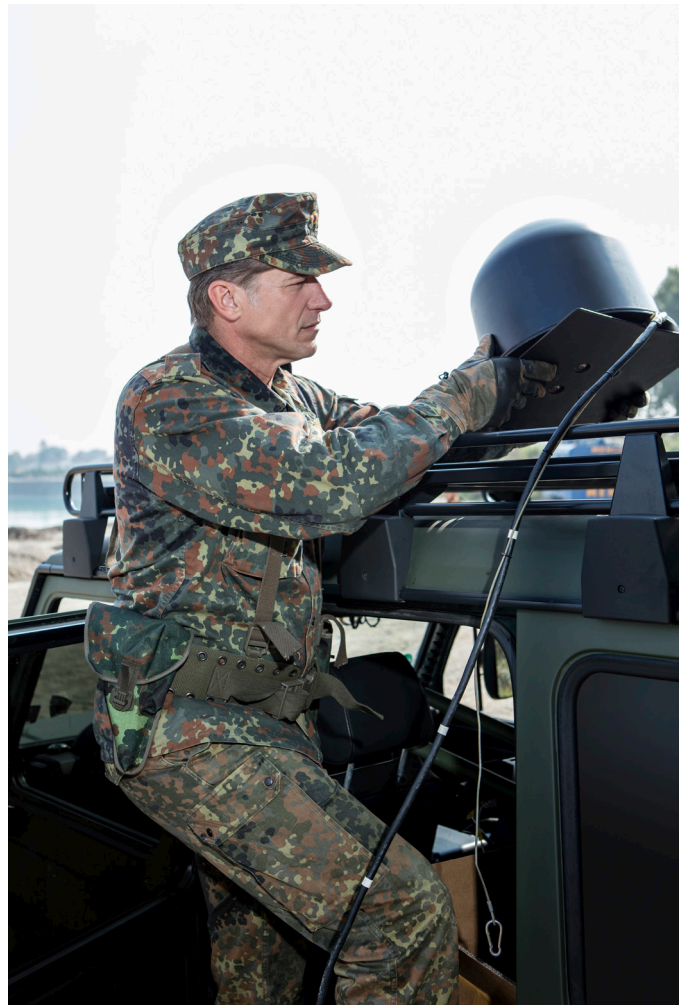
Automatic direction finding with Rohde & Schwarz compact DF antenna on a magnet mount (requires R&S®CS-DF option)
